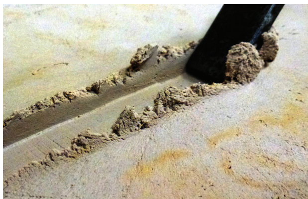
FIGURE 1: Ploughing of soft clay by a flat, inclined plate of narrow width.
