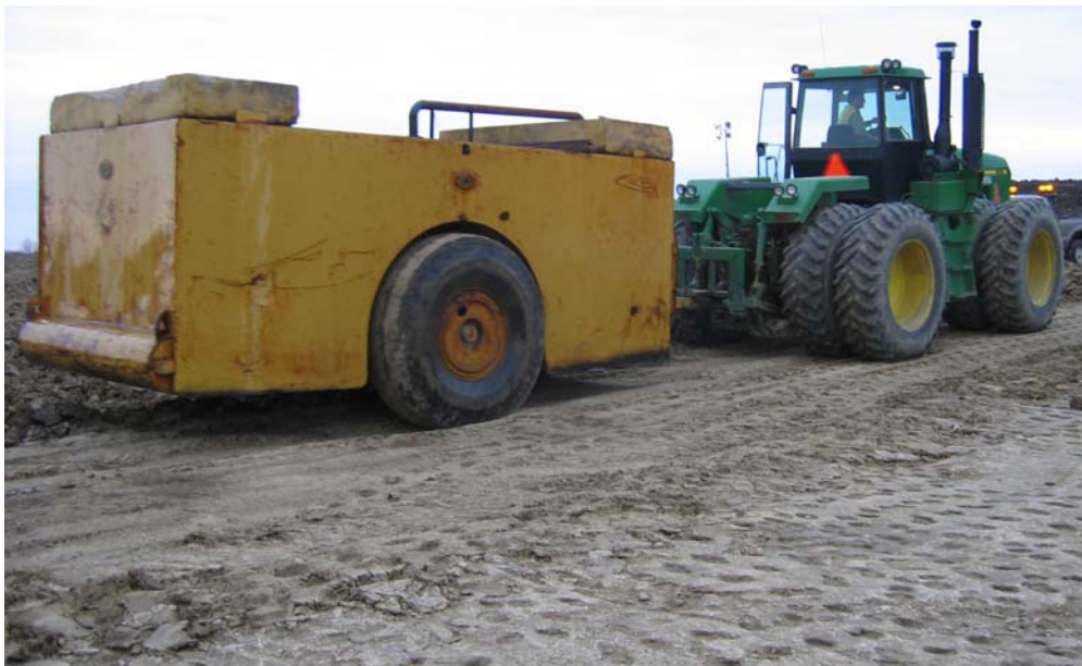
FIGURE 1 Example of test rolling device specified by the Minnesota Department of Transportation [2].
