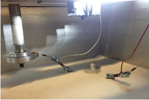
Fig. 16 Experimental setup showing the caisson model in the centrifuge box before testing with \alpha = 120^\circ .
